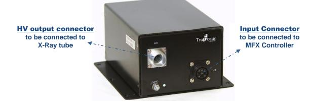
**MicroFocus HV Module** is a HV voltage multiplier (High Voltage Divider) and is designed in conjunction with TruFocus' MicroFocus Controller and MicroFocus X-Ray source to form a fully programmable MicroFocus X-Ray sub-system. MicroFocus Controller controls and monitors the output voltage and current of the MicroFocus HV Module.
